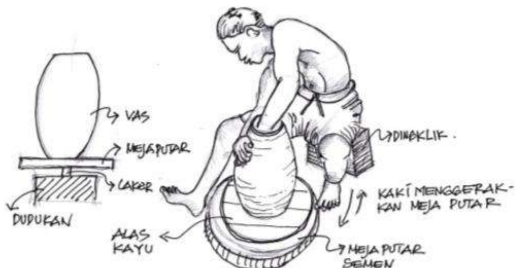
Figure 7. Foot turning technique
