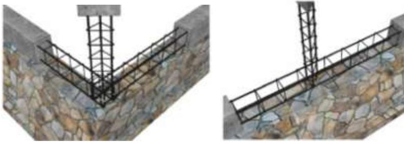
**Figure 2: The Triadic Column to Reduce the Building Structure Material**
